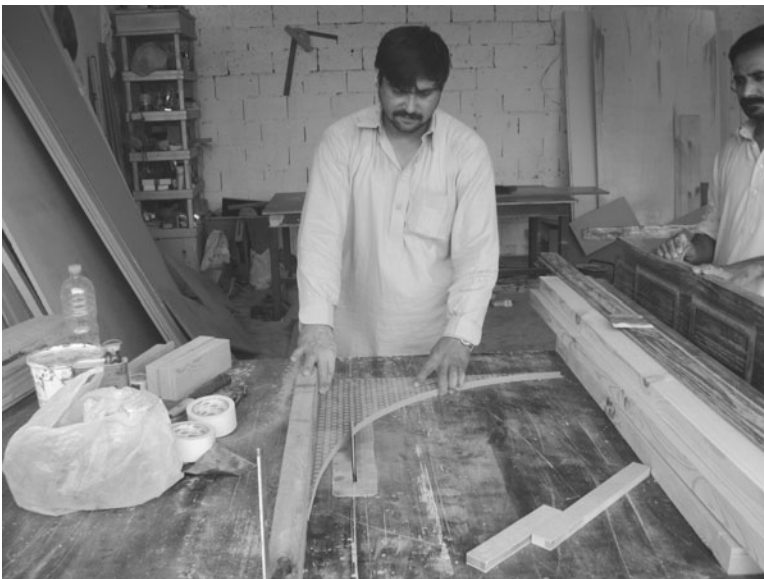
Figure 6.3 This worker is hand-feeding a piece of wood into a table saw with fingers, without a guard to protect his hand or eye protection. (Photograph by Seifeddin Ballal, King Faisal University, Saudi Arabia.)
