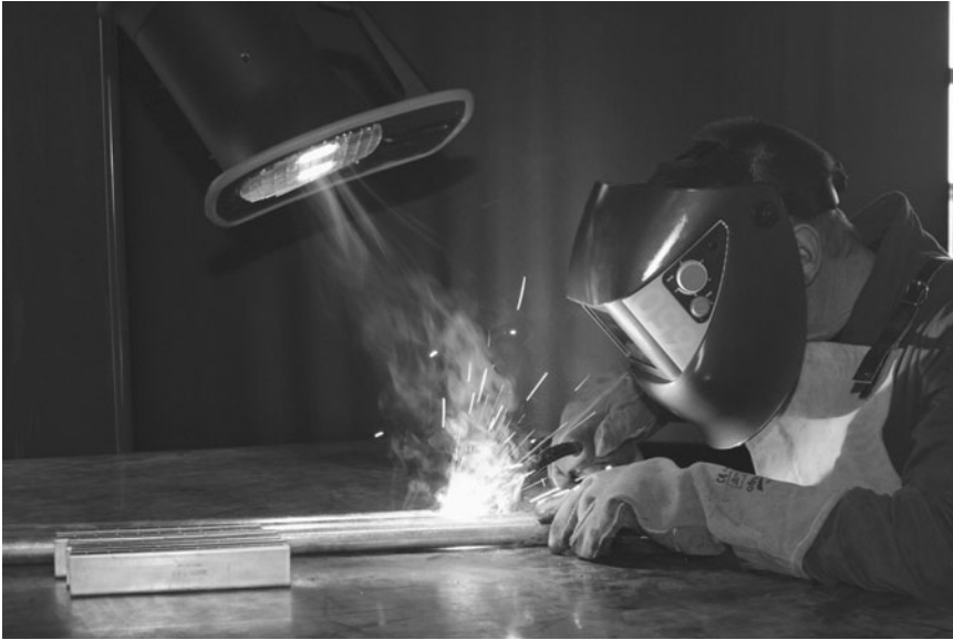
Figure 12.2 This local area exhaust ventilation duct system is designed specifically for welding operations. There is another example of this type of exhaust ventilation in Figure 8.2, the Kemper Exhaust Hood. (Photograph courtesy of the manufacturer, © Kemper America.)
