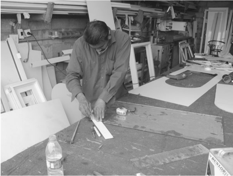
Figure 6.4 This worker is cutting glass with no protection for hands or eyes. (Photograph by Seifeddin Ballal, King Faisal University, Saudi Arabia.)
