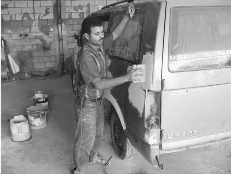
Figure 4.3 Automobile body work uses filler material consisting of fibrous glass, resin, talc, and styrene, which serves as a solvent and which evaporates. This results in exposure to styrene in a poorly ventilated area and in skin exposure, as in this garage in Saudi Arabia. (Photograph by Seifeddin Ballal, King Faisal University, Saudi Arabia.)
