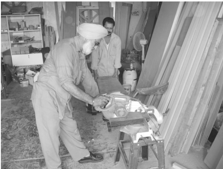
Figure 6.2 This worker has not properly secured the board he is sawing. (Photograph by Seifeddin Ballal, King Faisal University, Saudi Arabia.)
