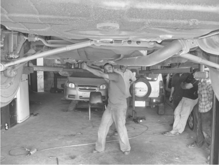
Figure 6.5 These workers are doing repairs under a car in a body shop under unsafe conditions: the frame holding up the car is not as secure as a hydraulic lift. (Photograph by Seifeddin Ballal, King Faisal University, Saudi Arabia.)
