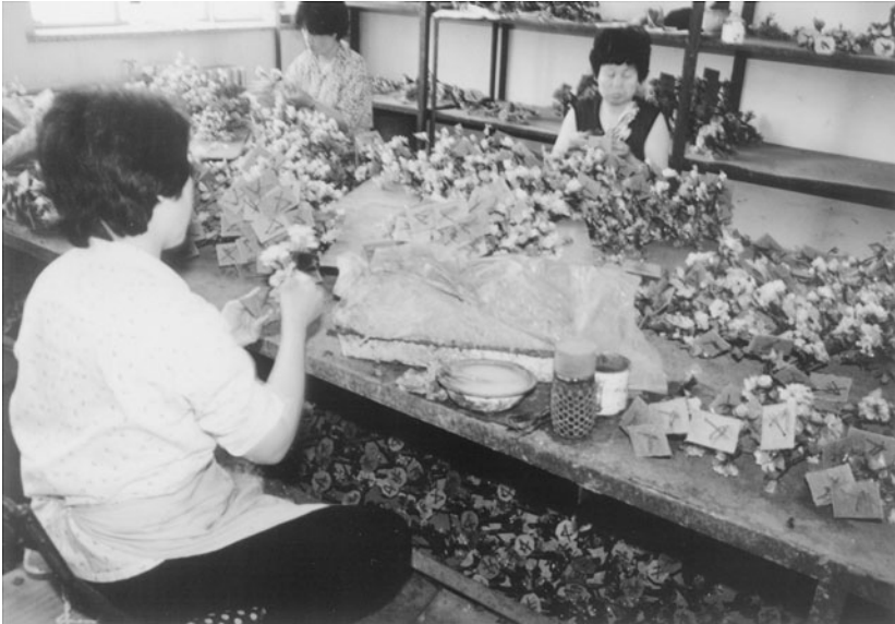
Figure 9.5 A factory (township enterprise) manufacturing glass flower arrangements, outside Beijing, in 1990. The glass contains high levels of lead, and the production of the glass leaves and flower petals exposed workers to high levels of lead; these workers are in the assembly area. (Photograph by Tee L. Guidotti, University of Alberta.)
