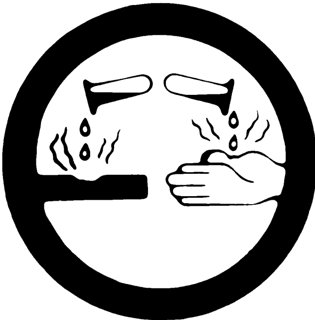
Figure 2.1 There is an international system of Chemical Safety Symbols used in most countries to identify chemical hazards; this is the symbol for a corrosive chemical that destroys materials and damages human tissue.
