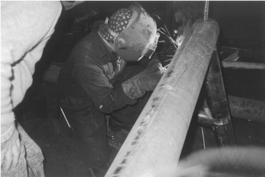
Figure 24.5 Arc welder welding a pipestand in Alberta (Canada) for use in an oilfield. (Photograph by Tee L. Guidotti, University of Alberta.)
