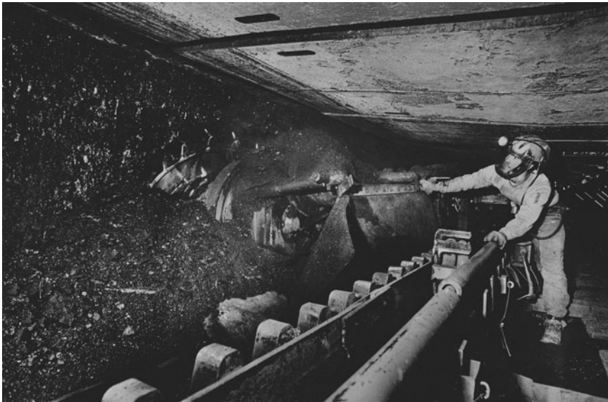
Figure 19.2 Coal mining in West Virginia (USA) is highly mechanized. A machine called a continuous miner digs out the coal from between layers of rock, and the coal is then brought out of the mine by a conveyor belt. Historically, coal mines have had many serious hazards, both for injury and for occupational disease, mostly coal workers' pneumoconiosis resulting from inhalation of dust. Note that this miner is wearing face protection and a light on his hard hat (helmet) and that the ceiling (called the "roof") is reinforced to prevent rock from caving in. (Photograph by © Earl Dotter, all rights reserved.)
