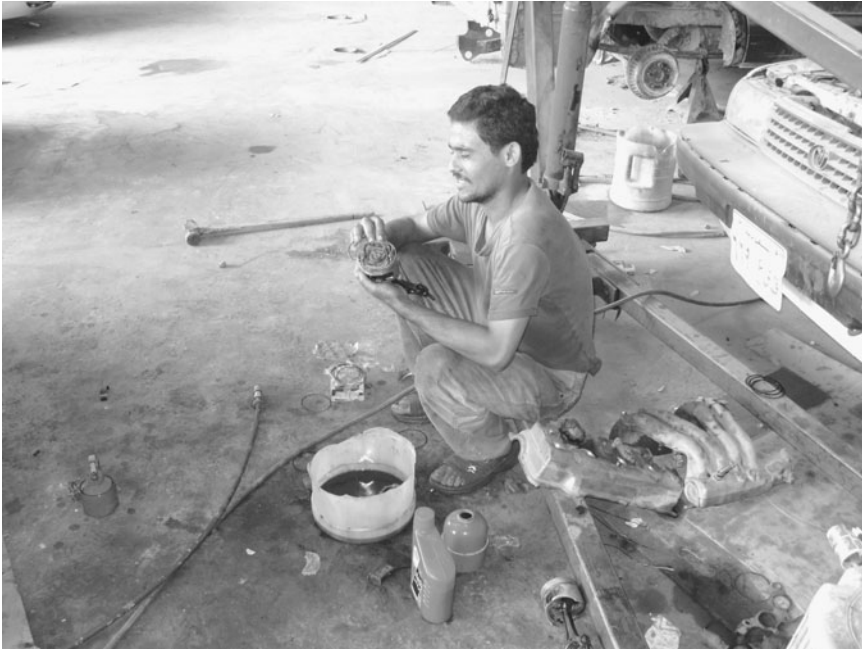
Figure 9.4 Cleaning automobile parts exposes this worker to solvents through skin absorption and through inhalation. (Photograph by Seifeddin Ballal, King Faisal University, Saudi Arabia.)
