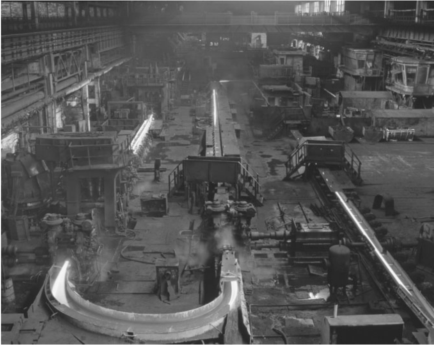
Figure 19.6 A continuous rolling steel mill in Ukraine, making pipe. (Photograph by Oleg Fedorenko, iStockphoto.)
