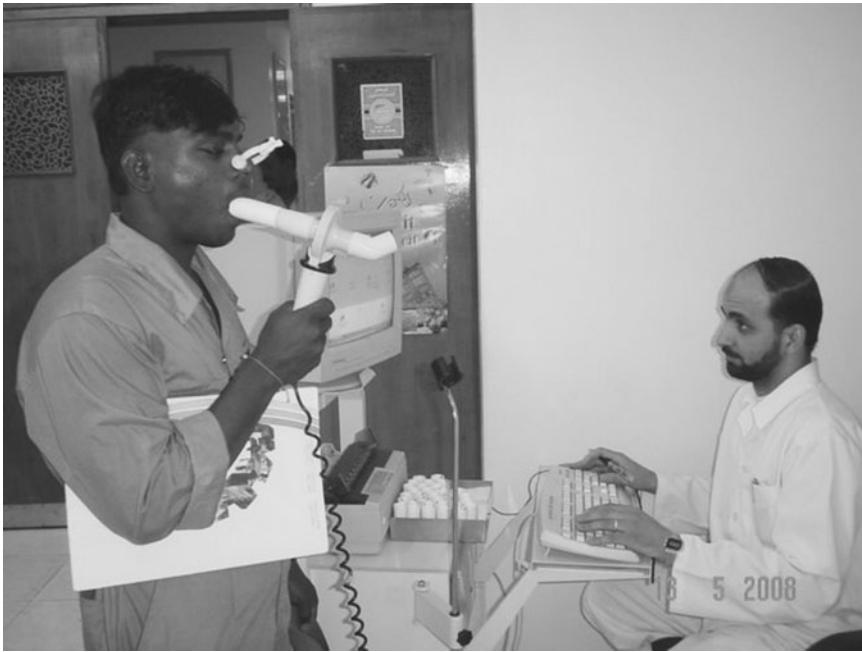
Figure 13.1 Pulmonary function testing is performed using a device called a “spirometer” that measures flow rates during breathing and the capacity of the lungs. Spirometry is a simple but extremely useful and reliable test of lung function. Spirometry alone is sufficient for screening purposes, but additional studies are usually performed for diagnosis of lung disease. (Photograph courtesy of Shuiaba Occupational Medical Centre, Ministry of Health, Kuwait.)
