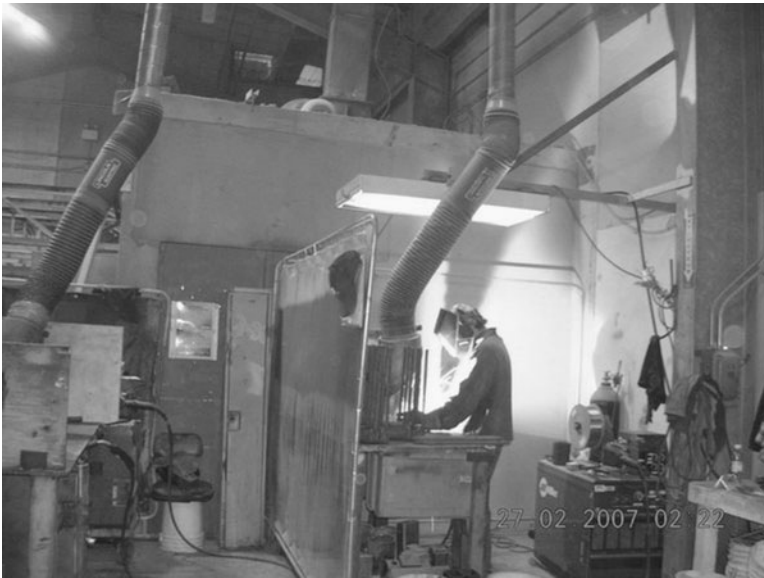
Figure 8.2 Arc welding generates intense radiation in the ultraviolet and visible light parts of the electromagnetic spectrum. The welder’s helmet has built-in eye protection against ultraviolet radiation, and the yellow curtain centered in the picture filters out ultraviolet radiation to prevent others in the shop from being exposed. Note also the moveable area ventilation system. (Photograph by Julietta Rodríguez Guzmán, Universidad El Bosque, Colombia.)
