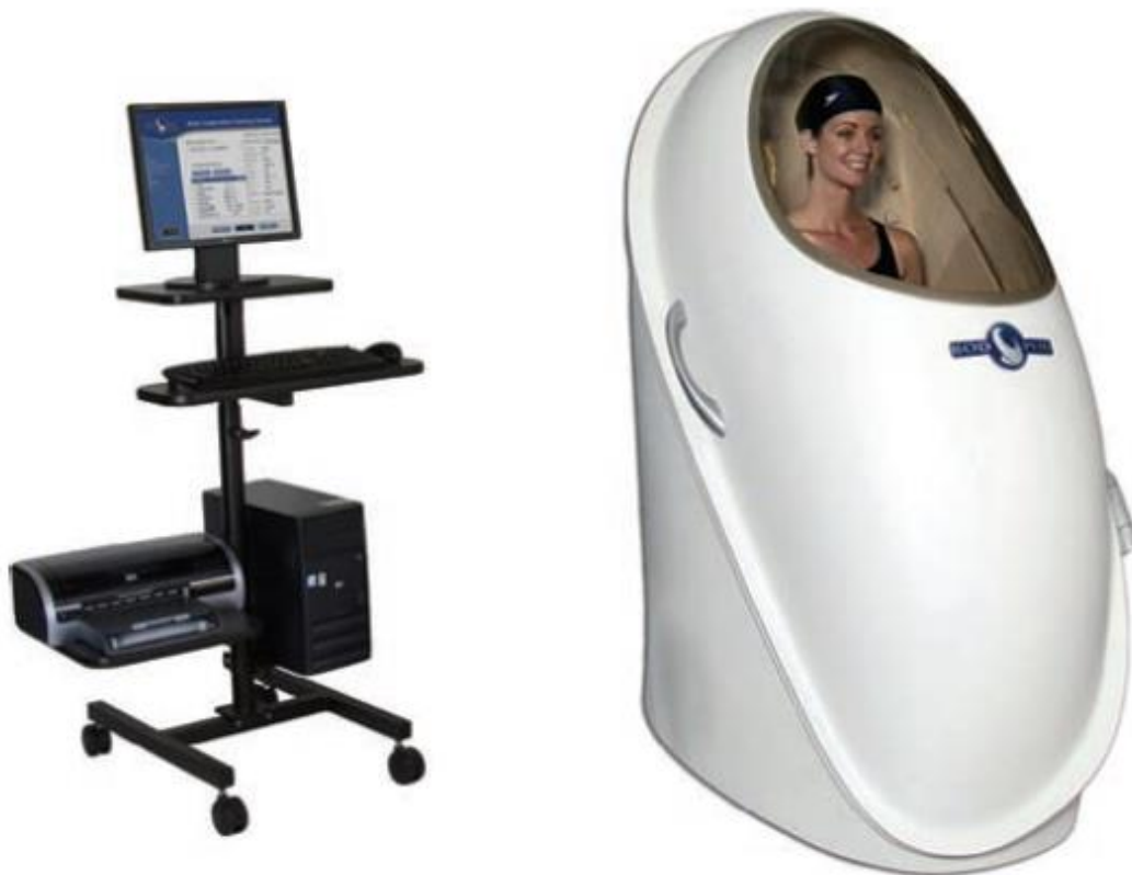
Figure 11-6. Air-displacement plethysmography uses differences in the volume of air in a sealed chamber to determine body volume. Once body volume is determined, equations similar to those used for hydrostatic weighing are used to calculate body density and other measures of body composition. (Photo courtesy of LifeMeasurement, Concord, CA.)
