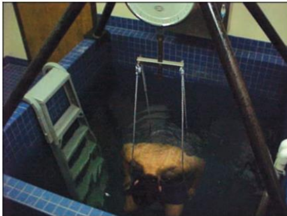
Figure 11-4. During hydrostatic weighing or densitometry, the person is completely submerged under water. As % fat increases, body volume increases, resulting in a greater displacement of water and so a decrease in underwater weight.
