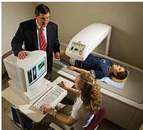
Figure 11-8. DEXA can be used to determine bone density and body composition. A major advantage of DEXA compared with other body composition methodologies is the ability to determine regional body composition and bone density.
