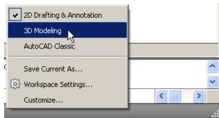
The 3D Modeling workspace provides easy access to 3D modeling and visualization tools via the AutoCAD ribbon. It also displays the tool palettes on the right side of the AutoCAD window.
