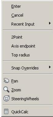
If you don't enter a value for the top radius, it assumes a value of zero and creates the cone with a sharp point. Also, keep in mind that, like a cylinder, the base and top of a cone don't necessarily mean that the base has to be on the bottom and the top has to be on the top. For now, I'll create the cone using a default top radius of zero and I'll snap to the center at the bottom of the cylinder to specify the height.
