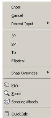
I'll use the default Center/Radius option and snap to the center and quadrant at the top of original cylinder. After specifying the base of the cone, the default option is to enter a value or pick a point to specify the height. However, there are additional options as well. A right-click menu (and the Command line) enable you to pick 2 points to determine the height, pick a point to specify the height and change the orientation at the same time, or enter a value for the top radius.
