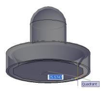
To specify the height, I'll drag the cylinder up and enter a value of 1.5. Since X-Ray mode is on, I can see the top edge of my new cylinder; reassuring me that I drew it in the right direction and at an appropriate size.
