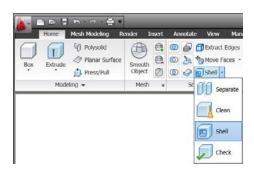
After you successfully launch the right Shell tool, you're prompted to select a 3D solid object and then you're prompted to remove faces. "Remove faces" doesn't mean it's going to remove faces from the object. It's giving the option to exclude faces from the shell operation. For example, when I performed a shell on the air hockey paddle, I selected the circular face at the bottom of the cylinder resulting in an open bottom.
